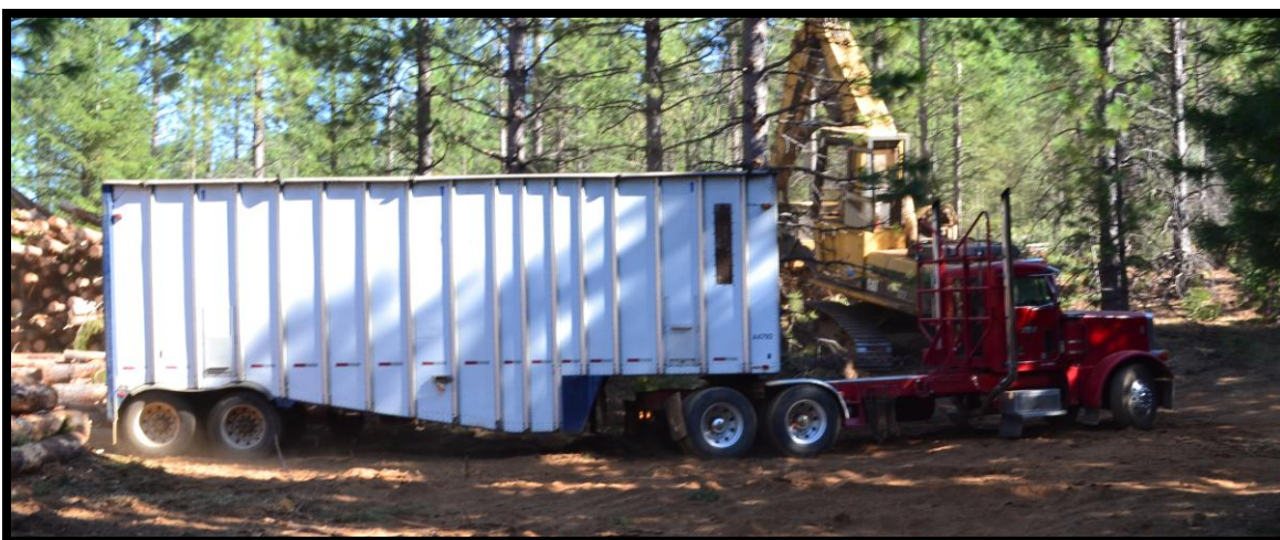
Figure 26. Short Trailer Maneuvering at the Landing in Preparation for Loading
